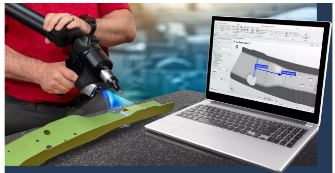
Laser scanning guided by CAD model in PolyWorks|Inspector
